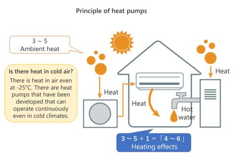
Air to Water (A/W) heat pump transfers heat from the outside air to water inside
