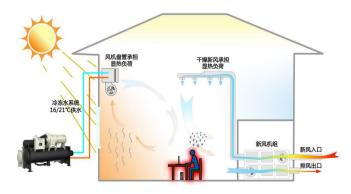
valve to meet the requirements of high temperature operation conditions and improve the efficiency of the compressor. The new high-efficiency water chiller which was developed based on the above technology causes the higher water supply temperature than indoor dew point temperature, has no risk of condensation, achieves efficient and reliable operation under the higher temperature conditions.
